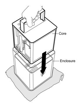
With a flat hand, press down on the latch until it locks into place. Firmly press the core to ensure it is fully secured within the enclosure.
